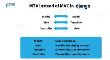
In MTV, the definitions of Model still remain the same that is, the Model contains the <u>logical file</u> <u>structure of the project</u> and is the middleware & data handler between database and view. The Model provides a definition of how the data formats as coming from the view so, it stores in the database and vice-versa, i.e., the retrieving information from the database transfers to the view in the displayable format.
